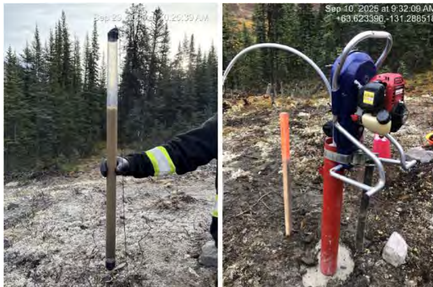
Figure 3 – Geotechnical investigations included the installation of 23 groundwater wells from which water quality and hydrology data will be collected to support PFS and Environmental Assessment work.
