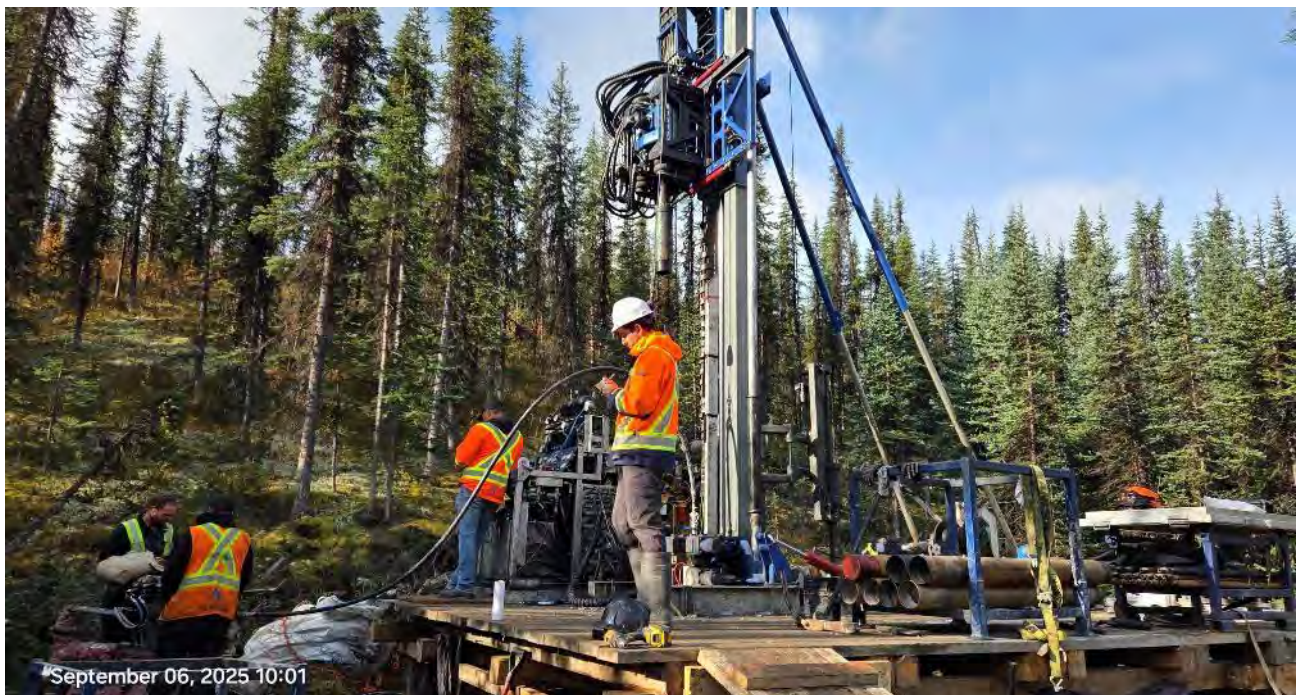
Figure 1 – Sonic drill rig setup near Snowline’s Valley deposit, Rogue Project. The Company drilled 51 sonic holes in 2025, characterizing surface materials around the Valley deposit and at various potential infrastructure sites to inform PFS work and de-risk project planning.
