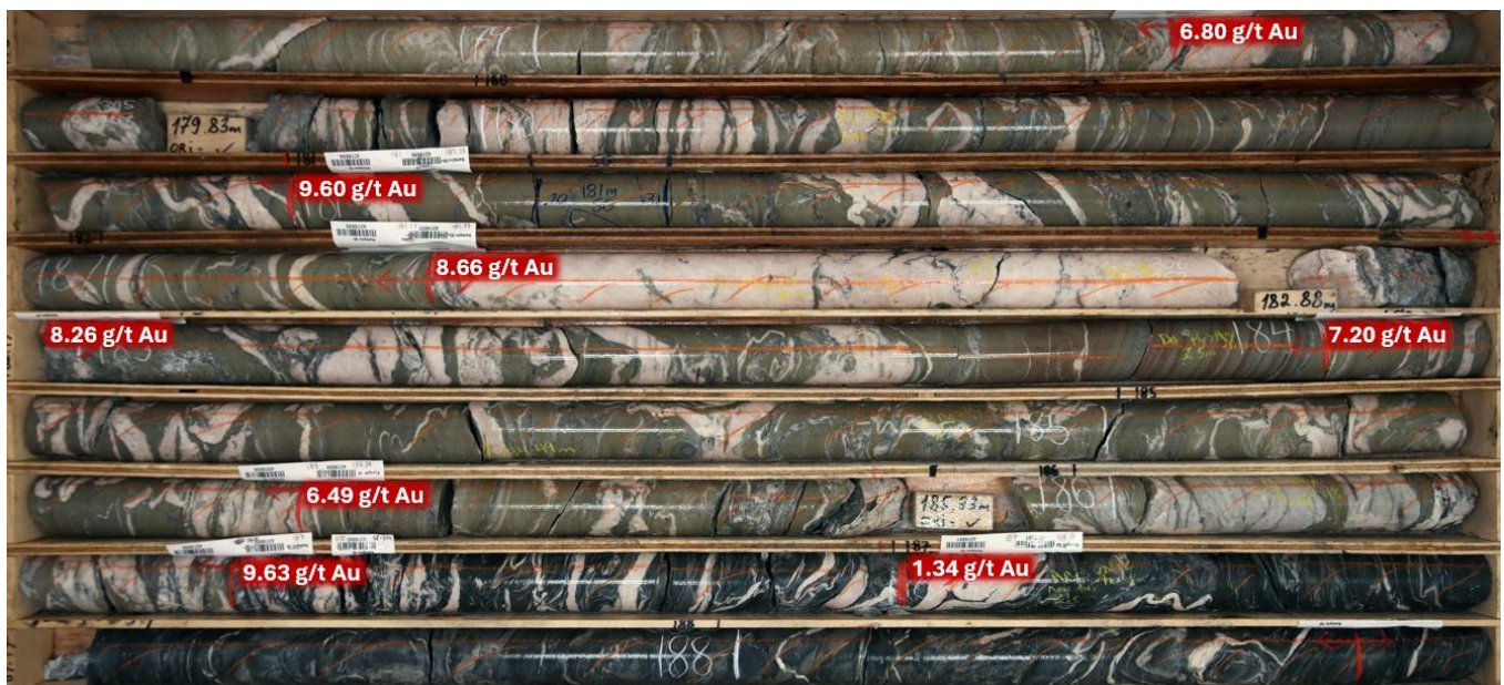
Figure 2 – J-25-037 drill core from 178.6 m to 188.6 m downhole, showing mineralized quartz-carbonate veins and surrounding mudstones. Assay values for individual samples are highlighted in red, with red vertical lines on the drill core denoting sample boundaries.
