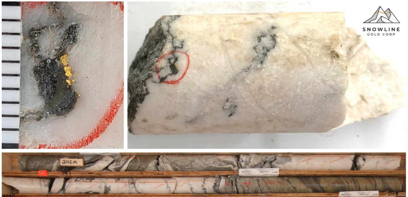
Figure 5 – Visible gold in a steeply dipping E-W quartz-carbonate vein from J-24-031 at 246.5 m downhole. The vein material averaged 4.3 g/t over 1.5 m from 246.0 m downhole, at the base of a broader zone averaging 2.64 g/t Au over 5.0 m from 242.5 m downhole. Core diameter is 5.1 cm, with millimetres denoted by the scale bar in the top left image.
