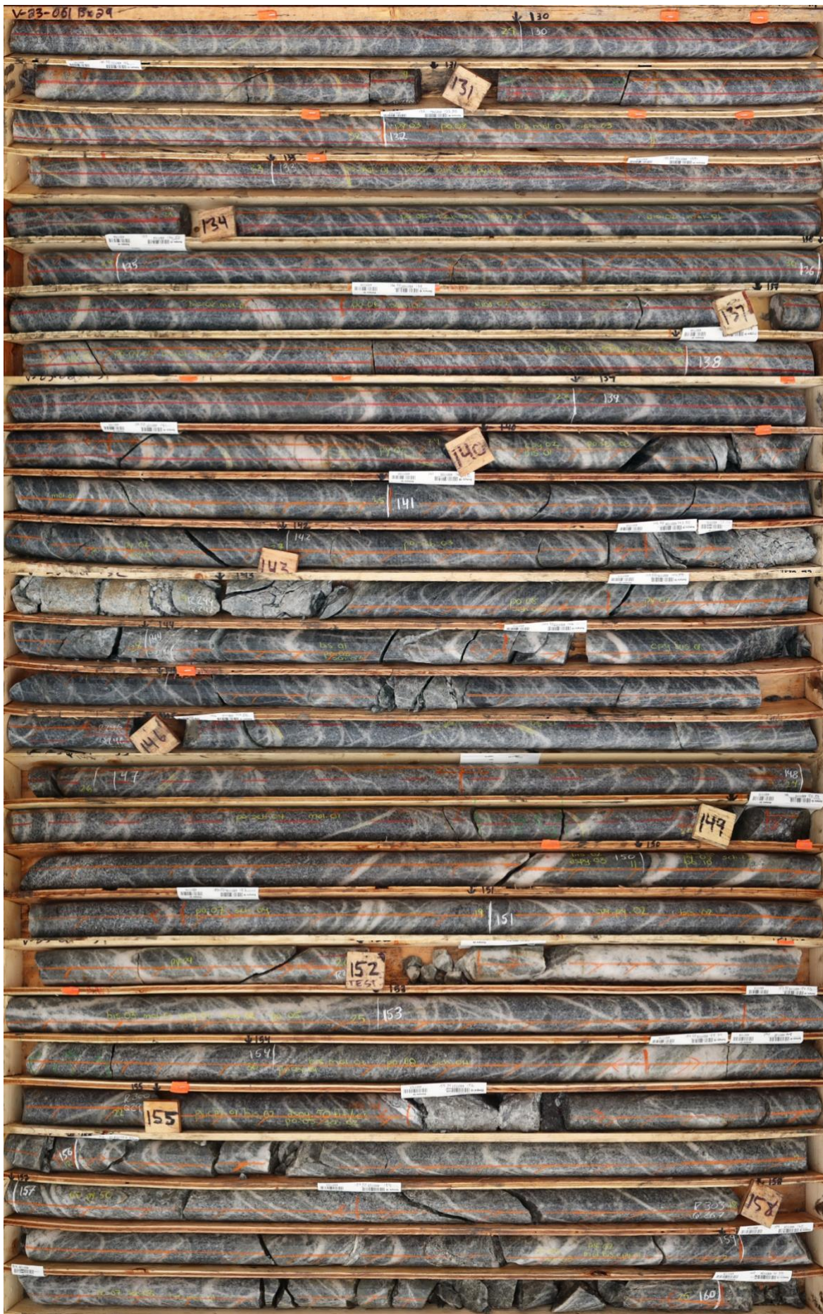
Figure 3 – High quartz vein density observed in V-23-061, from 129.3 m to 160.0 m downhole, as seen in a September 11, 2023 news release. This 30.7 m downhole interval averages 5.87 g/t Au and includes the top of a 47.5 m interval averaging 6.47 g/t Au from 149.0 m downhole. Orange flagging marks instances of trace visible gold. Multiple generations of quartz veins can be seen cutting the core at different orientations. NQ2 sized drill core shown is 5.1 cm in diameter.
