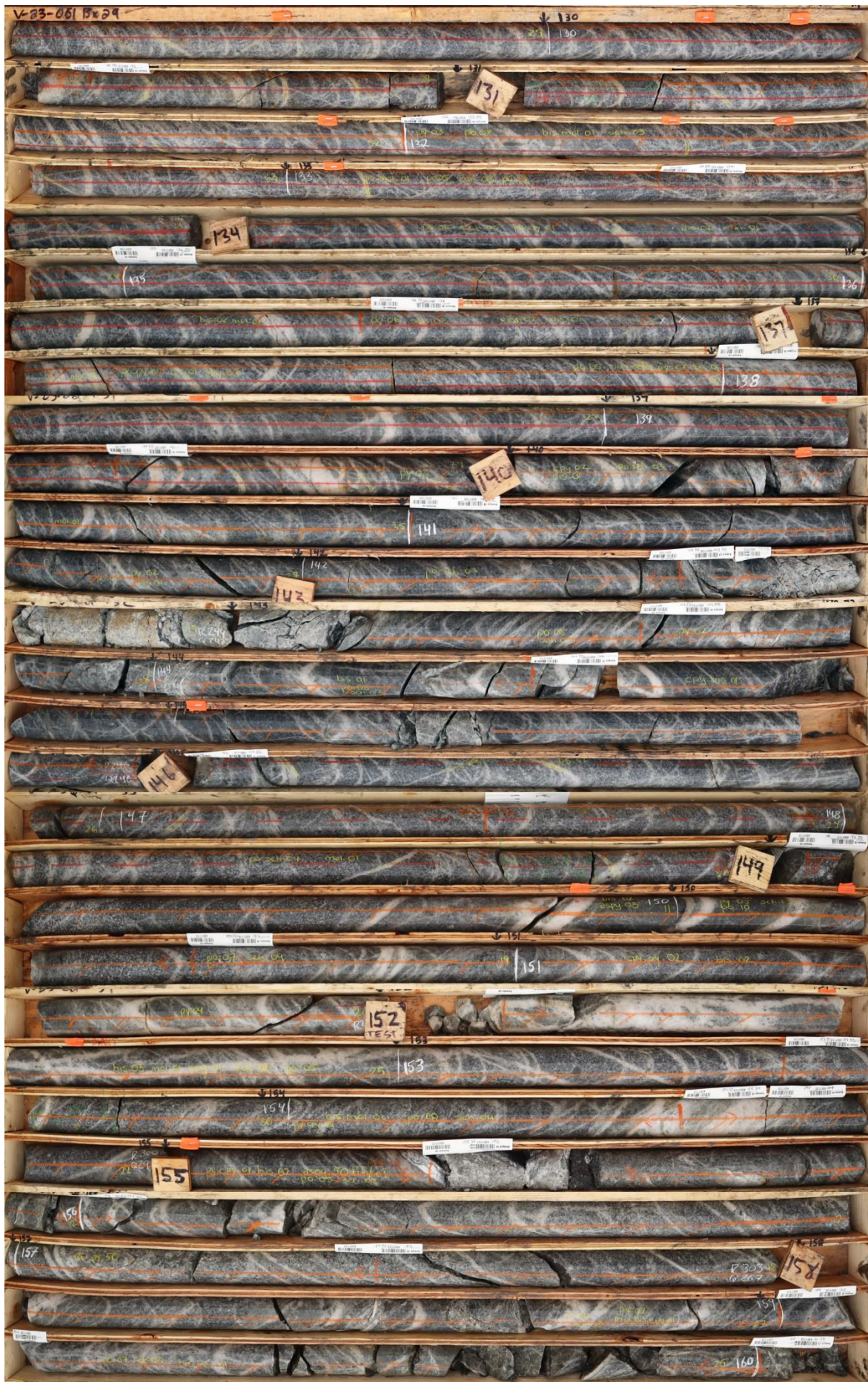
Figure 5 – High quartz vein density observed in V-23-061, from 129.3 m to 160.0 m downhole in a composite photo. Orange flagging tape marks instances of trace visible gold observed during logging. Multiple generations of veins can be seen cutting the core at different orientations. NQ2 sized drill core shown is 5.1 cm in diameter. The above vein densities are not representative of the entire hole. Assays are pending for this section and the remainder of the hole.
