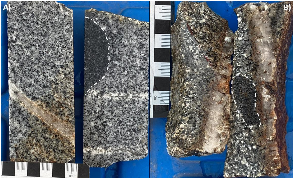
Figure 4 – Intrusive host and veining style at Valley (left) and Cujo (right). Coarse grained granodiorite with fine-grained biotite rich xenoliths (outlined by white dashed lines). Sericite-chlorite alteration and quartz-calcite-bismuthinite-scheelite veins. A) Core samples from hole V-23-036 at the Valley target, 5 to 8 meters depth. B) Surface sample from the Cujo target.
