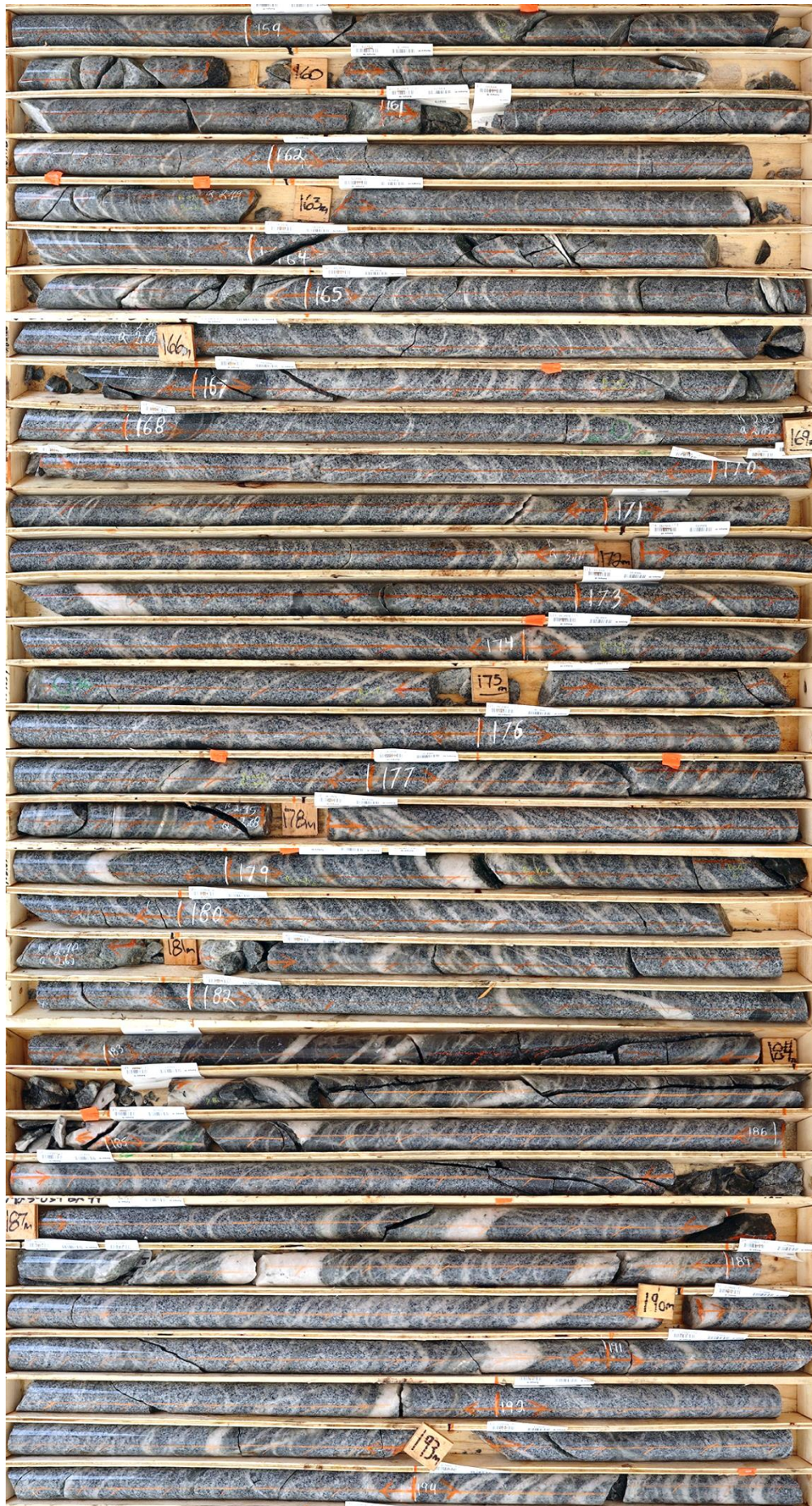
Figure 2 – Quartz vein mineralization in V-23-034, from 158.7 m to 194.5 m downhole, a subset of a larger run of similar moderate to high quartz vein density beginning at bedrock surface. The core shown averages 4.32 g/t Au. It sits atop a 121.4 m interval averaging 4.12 g/t Au from 158.0 m downhole, with 80% of assays by distance returning >2 g/t Au. True widths have not been determined.
