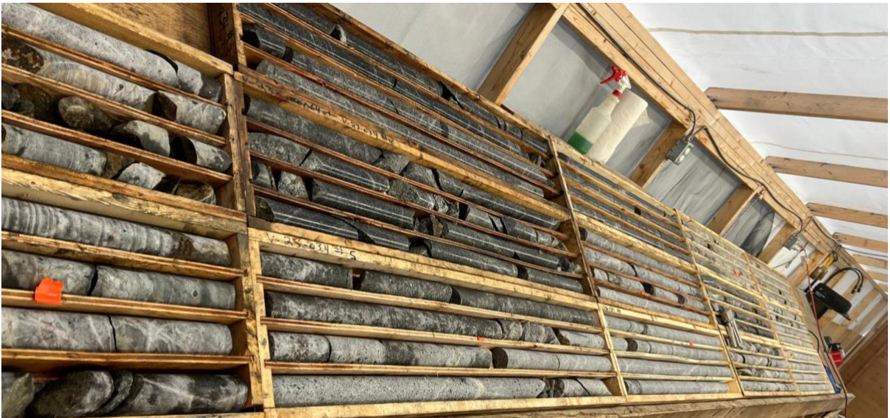
Figure 1 – The first delivery of core from the rigs in 2023, from hole V-23-34 on the Rogue Project's Valley target, in Snowline's newly-expanded core shack. Visible gold was observed within sheeted quartz veins in 10 of the 14 boxes during preliminary logging, along with intrusive breccia textures and at least 3 generations of quartz vein at moderate overall densities. Orange flagging tape marks the locations of visible gold, with the first encountered at 12 m downhole.
